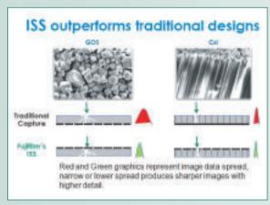
This revolutionary new detector also features Fujifilm's patented ISS (Irradiation Side Sampling) which provides ultra-sharp imaging with superior dose efficiency. This exclusive design captures the x-ray image from the incident/patient side of the detector, in contrast to traditional designs which capture the image below/behind the scintillator layer. FDR D-EVO™ Wireless captures the sharpest detail for both strong and weak penetrating x-rays, making the finest details and hairline
